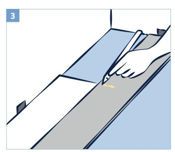
Continue connecting the first row until you reach the last full plank. Fit the last plank by rotating the plank 180° with the pattern side upward, place beside row. Measure and mark, then using a ruler and utility knife, score the plank and snap off. Attach as described above.
