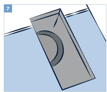
Door frames and heating vents also require expansion room. First cut the plank to the correct length. Then place the cut plank next to its actual position and use a ruler to measure the areas to be cut out and mark them. Cut out the marked points allowing the necessary expansion distance on each side.
