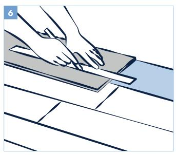
To fit the last row, lay a plank on top of the previous row. With the tongue to the wall, lay another plank upside down on the one to be measured and use it as a ruler. Don't forget to allow room for spacers. Cut the plank and attach into position.
