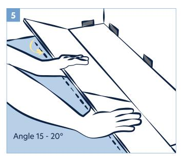
To attach the second row to the first row, tilt and push the side tongue into the side groove of the first panel at an angle of approx. 15-20 degrees. Lower and click into place lining the edges up carefully. Continue laying remaining planks in this manner.
