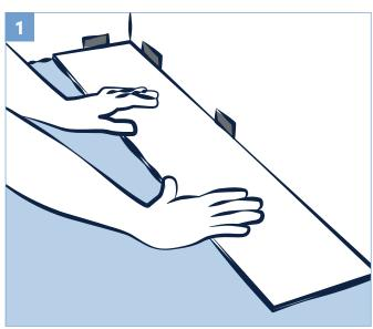
Start in a corner by placing the first plank with the tongue side facing the wall. Use spacers along each wall to maintain an expansion space of 8-12 mm ( $^5/_{16}$  in -  $^3/_8$  in) between the wall and the flooring.
