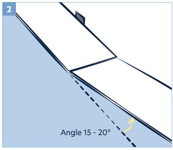
To attach the second plank, insert the end tongue into the end groove of the very first plank at an angle of approx. 15-20 degrees. When lowered, the plank will click into place. Line up edges carefully. The planks should be flat to the floor.
