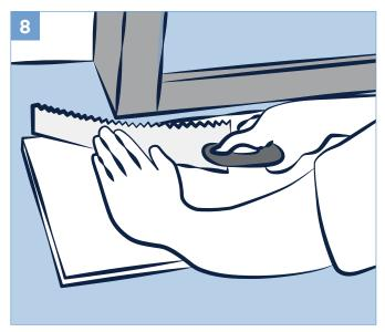
You can trim door frames by turning a plank upside down and using a handsaw to cut away the necessary height so that planks slide easily under the frames.
