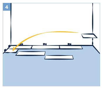
Begin the next row with the off-cut piece from the previous row to stagger the pattern. Pieces should be a minimum of 20 cm (8 in) long and joint offset should be at least 40 cm (16 in).
